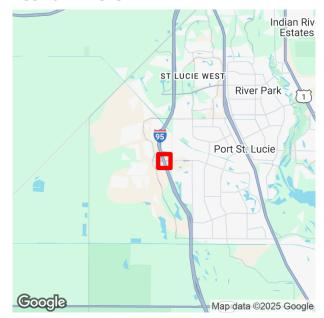
Project Description: INTERCHANGE - ADD LANES Extra Description: GATLIN BLVD AT NORTHBOUND & SOUTHBOUND OFF-RAMP INTERSECTION SHORT TERM IMPROVEMENTS: A)ADD A THIRD LEFT AND TRIPLE RIGHT TURN LANES ON SB OFF-RAMP WITH MINOR WIDENING TO RECEIVING LANES ON GATLIN BLVD. B) ADD THIRD LEFT TURN LANE AND DUAL RIGHT TURN
