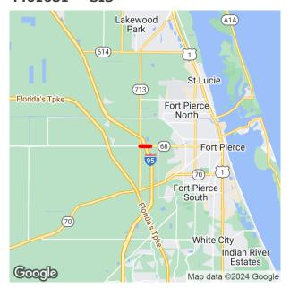
Project Description: INTERCHANGE - ADD LANES Extra Description: ADD EB RIGHT TURN LANE FROMOM ORANGE AVE/SR-68 TO I-95 SB ON-RAMP & ADD WB RIGHT-TURN LANE FROM ORANGE AVE/SR-68 TO NB KINGS HWY/SR-713 NB & WB PROTECTED RIGHT TURN PHASES TO BE ADDED AT INTERSECTION OF ORANGE AVE/SR-68 AND KINGS HWY/ SR-713 EB TO SB ON-RAMP ENTRANCE TO BE RELOCATED TO THE EXISTING SIGNALIZED INTERSECTION FOR THE WB TO SB (SEE WP45)
