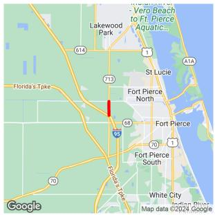
Project Description: ADD LANES & RECONSTRUCT Extra Description: 2017 TPO PRIORITY #4 WIDENING 2 TO 4 LANES, PD&E UNDER 230256-5, DESIGN & ROW UNDER FM# 438379.1 Lead Agency: MANAGED BY FDOT County: ST. LUCIE From: NORTH OF I-95 OVERPASS To: SOUTH OF ANGLE RD Length: 0.97 Phase Group: CONSTRUCTION
